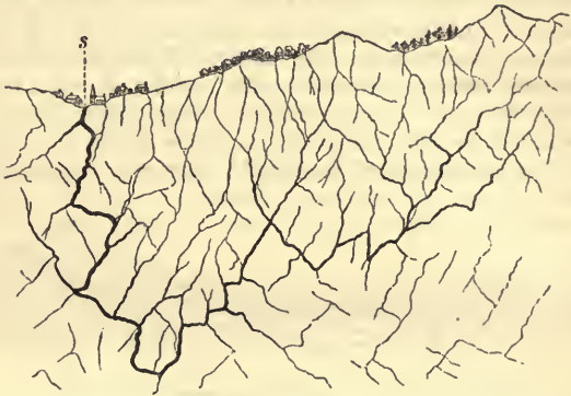
FIG. 48.—Section to show the intricate underground drainage which issues in a deep-seated spring. The numerous joints and cracks in the rocks lead the water at last into a main channel, by which it reascends to the surface as a spring at s .
